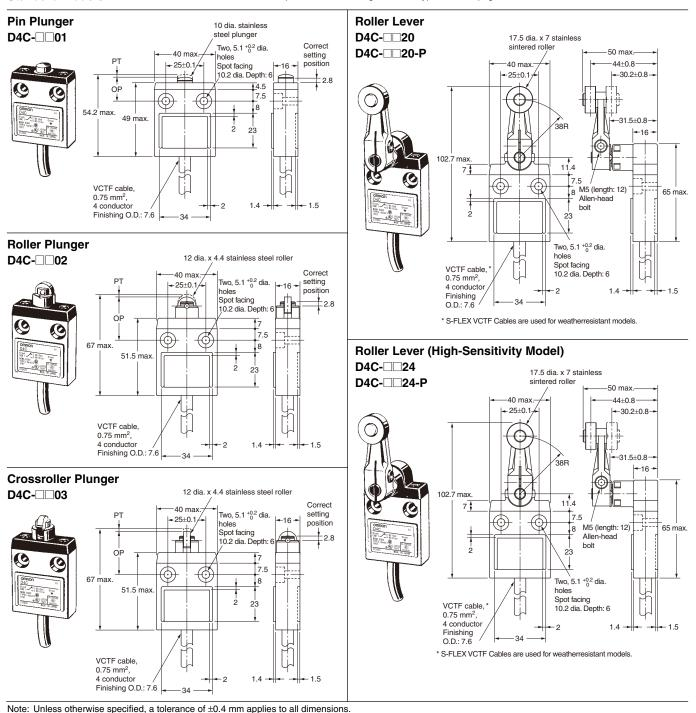
Model D4C-020 D4C-024 D4C-001 D4C-002 D4C-003 Operating D4C-020-P D4C-024-P characteristics Operating force OF max. 11.77 N 11.77 N 11.77 N 5.69 N 5.69 N Release force RF min. 4.41 N 4.41 N 4.41 N 1.47 N 1.47 N PT Pretravel 1.8 mm 1.8 mm 1.8 mm 25° 10°±3° max. Overtravel ОТ 3 mm 3 mm 3 mm 40° 50° min. Movement Differential MD max. 0.2 mm 0.2 mm 0.2 mm 3° 3° Operating Position OP 15.7±1 mm 28.5±1 mm 28.5±1 mm --------
